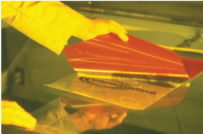
Reflex SR, applied using the indirect process, is available in rolls and custom cut sheets. Reflex SR is manufactured without the use of solvent-based materials.
