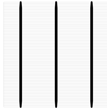
Figure 3. Grid design: 72 lines at 60µm each line with 1.5mm-wide busbars.
